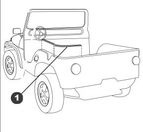
CJ5 Windshield Adjustment: If necessary, loosen the two screws in the Windshield Clamps at the base of the windshield on each side of the vehicle. Adjust the windshield forward or back, use a shim if needed to position the windshield, and tighten the screws.
